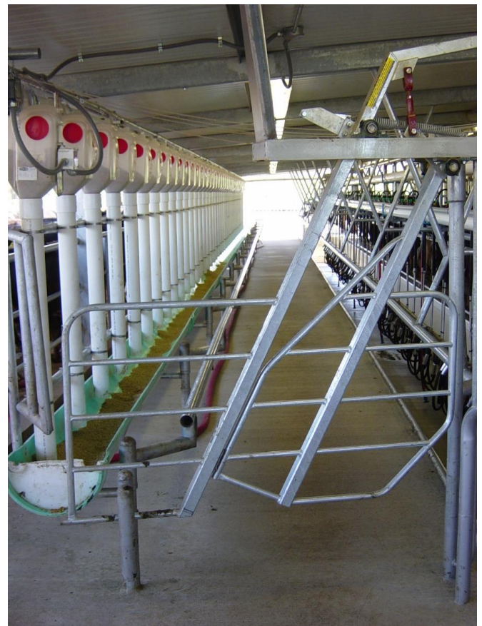
Figure 2. Swing parlor allows quicker milking.
